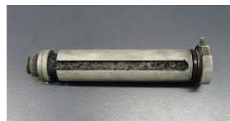
Immerse into Rust Remover A-310 with ultrasonic cleaner
