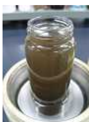
Immerse into Rust Remover A-310 with ultrasonic cleaner
